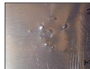
shot 5 spall witness plate rear
